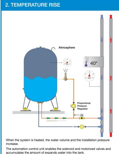
The air in the tank and the decomposed oxygens in the water throughout the
