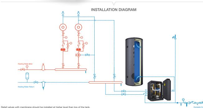
Thus it is protected against high temperature and calcification and it is not necessary to discharge the tank when working on the relief valve.
